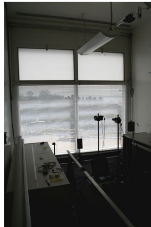
Interior view of test room with translucent panel in the upper daylighting zone and a conventional venetian blind in the lower view zone. Photo: LBNL.
