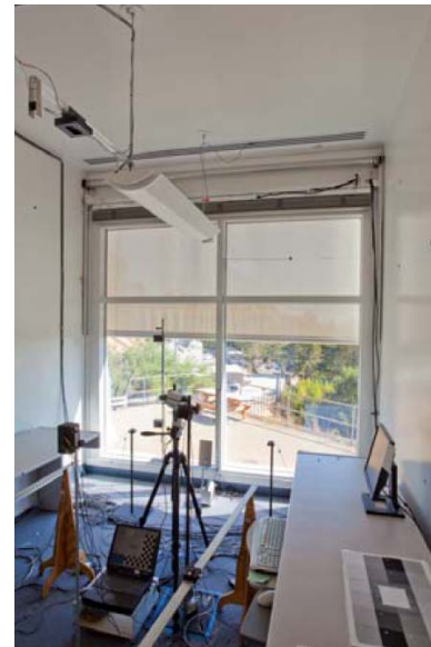
Interior view of an automated exterior roller shade with 3%-open, light gray (both sides), basketweave fiberglass/ PVC fabric. The shade could be set to an almost fully raised height for an unobstructed view out, but the bright sky may cause glare discomfort.
