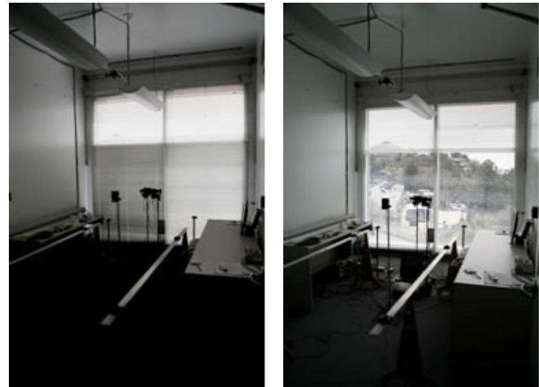
Interior view of test room with zoned blind. Left: upper slats are set to admit daylight and lower slats block sun. Right: lower slats are set to permit view out and upper slats are slightly closed. Photos: LBNL.
