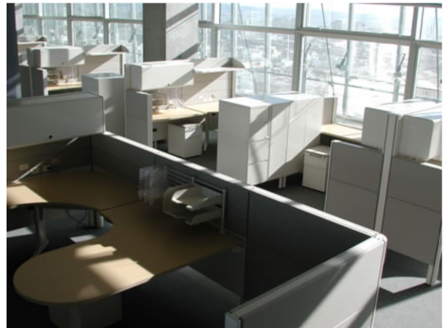
In this building, a 50%-open exterior metal scrim was assumed to be sufficient to control direct sun –after the occupants moved in, interior shades had to be installed to address complaints of thermal and visual discomfort. Photo: LBNL
