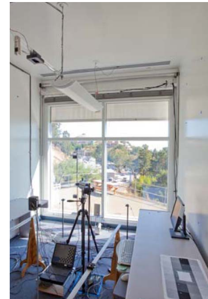
Interior view of an automated exterior roller shade with 3%-open, light gray (both sides), basketweave fiberglass/ PVC fabric. The shade could be set to an almost fully raised height for an unobstructed view out, but the bright sky may cause glare discomfort.
